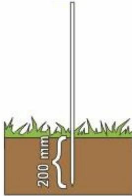
**Insert fibreglass stake and tap until firm.**
