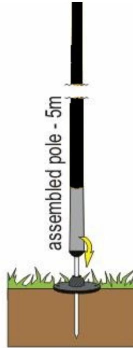
**Slowly slide assembled pole onto stake and position on Grounder.**
